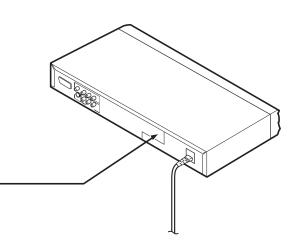
The rating plate and the safety caution are - on the rear of the unit.
